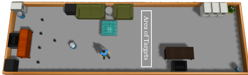
(A) A simulation environment with dynamic obstacles. The trash acted as an unexpected obstacles; the person acted as a moving obstacle. The team was assigned a mission to navigate to the Area of Targets.
